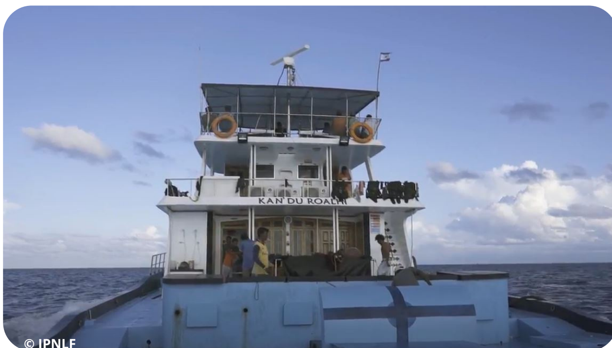
© IPNLF Vessel 'Kan'du Roalhi' with a Kuruno bird radar installed at the top of the vessel. The radar rotates and detects flocks of birds to assist fishers in locating schools of tuna
