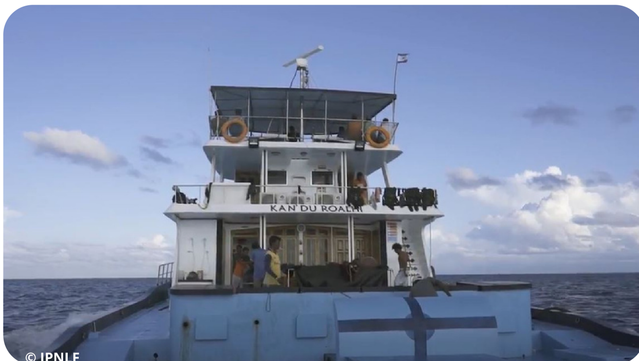
Vessel 'Kan'du Roalhi' with a Kuruno bird radar installed at the top of the vessel. The radar rotates and detects flocks of birds to assist fishers in locating schools of tuna
